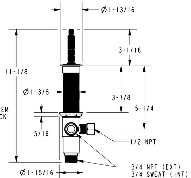
DIMENSIONS ARE IN INCHES AND AN APPROXIMATION OF A TYPICAL INSTALLATION
