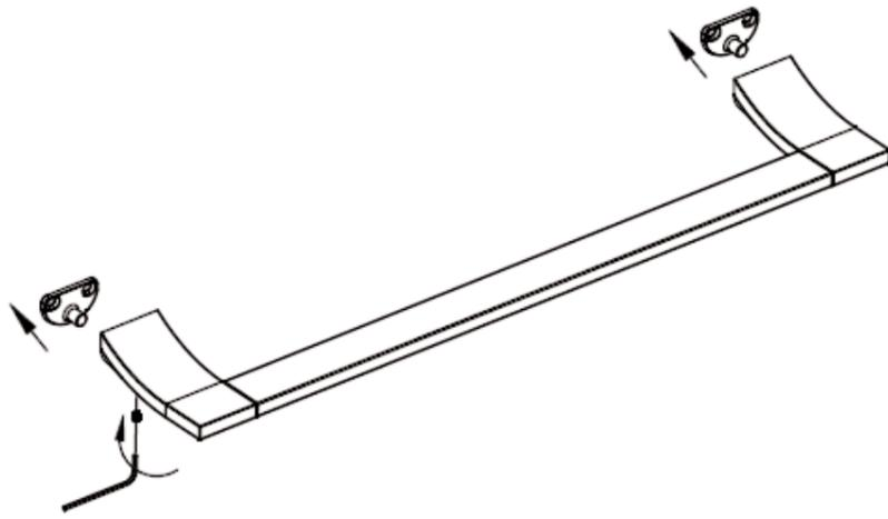
② ALIGN MOUNTING BRACKETS AND MARK LOCATION
