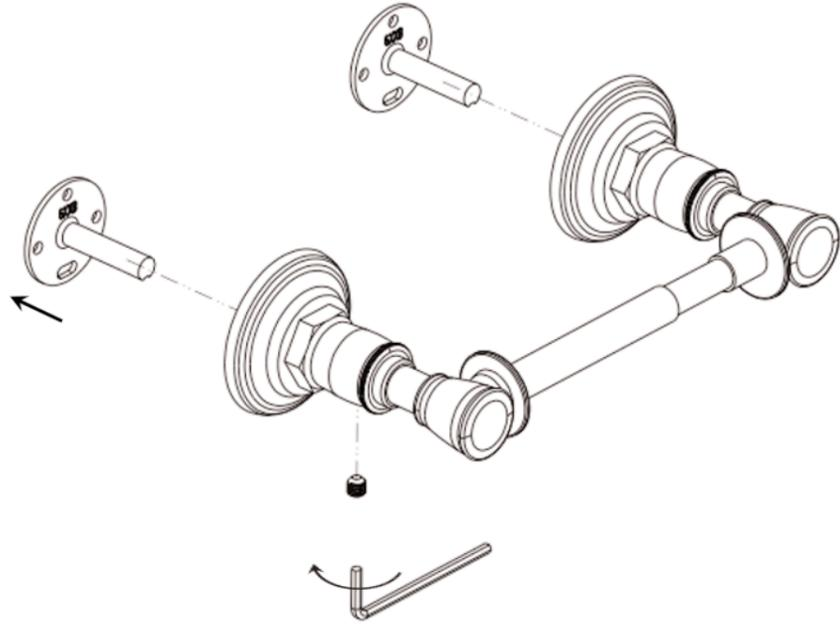
② ALIGN MOUNTING BRACKETS AND MARK LOCATION
