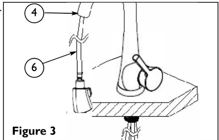
Do **NOT** remove the zip tie and ensure the hose does not rub against the hot/cold supply lines.
