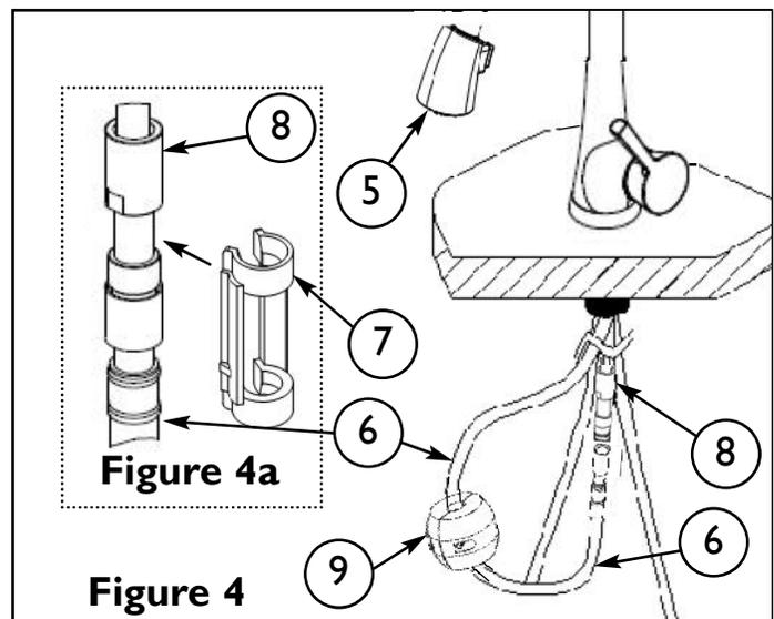
7. Connect HOSE (6) to valve outlet (8). See Figure 4. Attach CLIP (7) to the connection between HOSE (6) and OUTLET (8). See Figure 4a.
