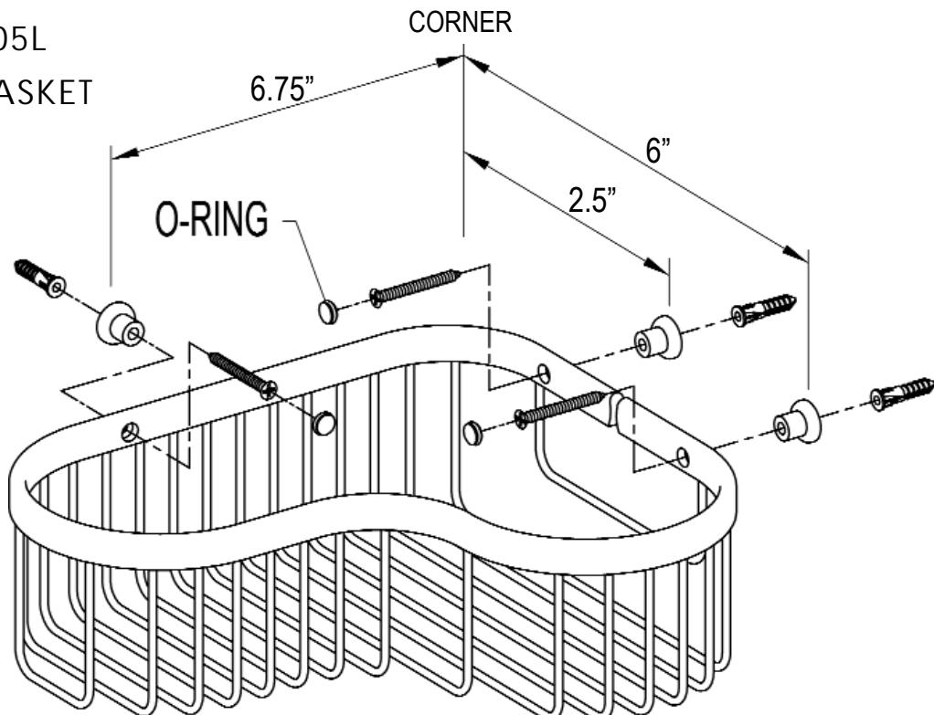
TO PREVENT LOSS OF SMALL PARTS, COVER DRAIN BEFORE BEGINNING.
