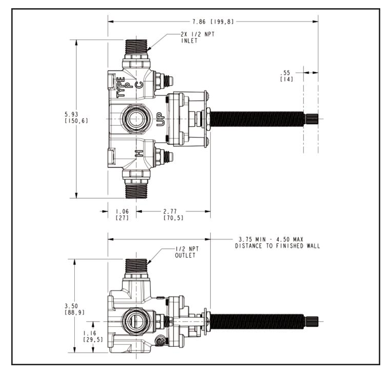
All Threaded Connections are 1/2" NPT Dimensions are in Inches and Approximation of a Typical Installation
