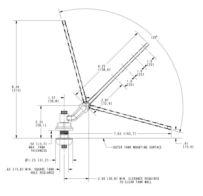
TANK LEVER MECHANISM 6-505
