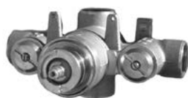
1-540 3/4" Thermostatic Rough-in Valve Flow rate of 18 gallons per minute at 60 PSI. Factory calibrated comfort setting at 100-deg F, built-in check valves with service stops. IAPMO Listed. Meets ASSE Standard 1016.
