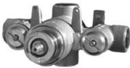
1-540 3/4" Thermostatic Rough-in Valve Flow rate of 18 gallons per minute at 60 PSI. Factory calibrated comfort setting at 100-deg F, built-in check valves with service stops. IAPMO Listed. Meets ASSE Standard 1016. MUST USE WITH SEPARATE STOP/VOLUME CONTROL
